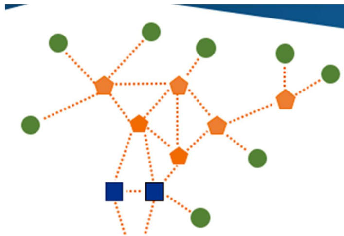
Figure 1: Diagram of a mesh network.
